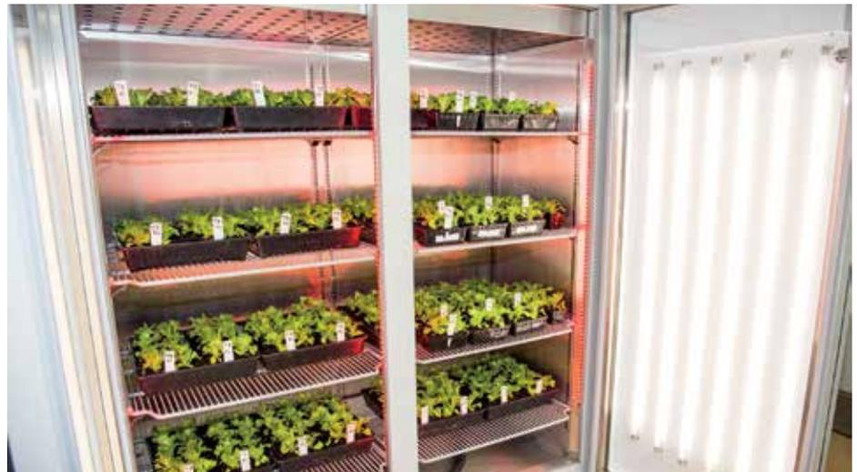
*A new Climatron plant growth cabinet is assisting the Peracto team to control the environment in research trials.*
